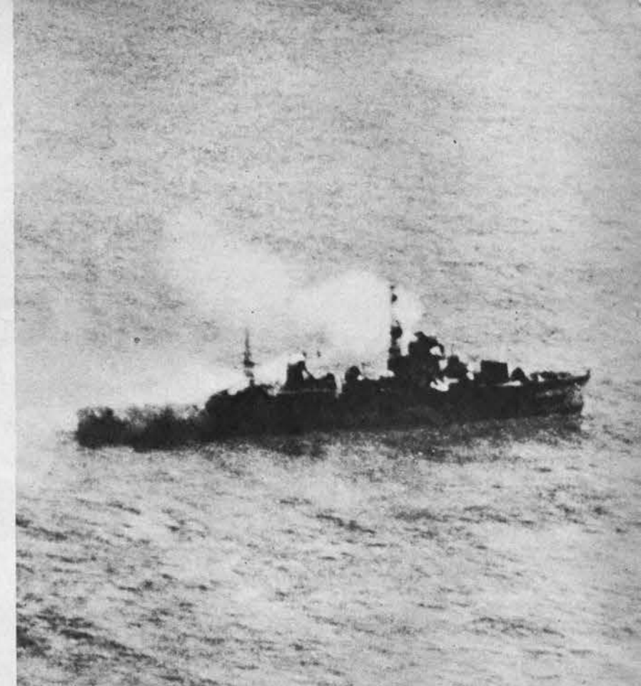
New destroyer escort is classified DE UN-1. Set well aft, stack is widely separated from the bridge structure which bristles with AA.
